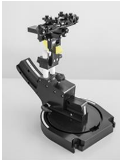
Device holder supplied by SPEAG
