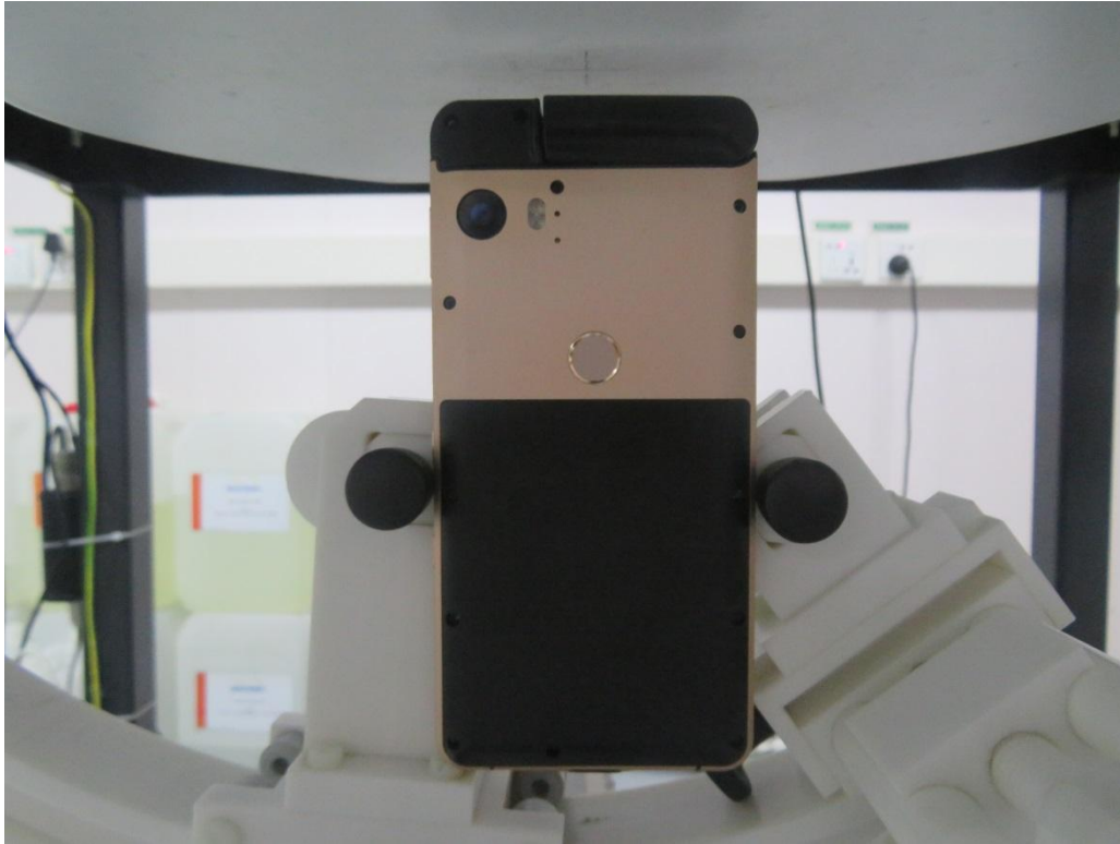
10mm body-worn Bottom Side Setup Photo (hotspot)
