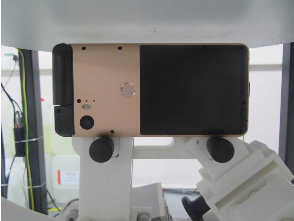
10mm body-worn Right Side Setup Photo (hotspot)
