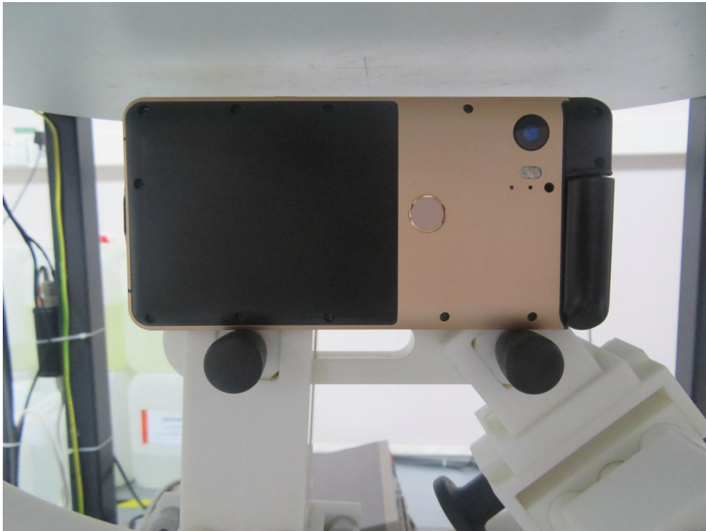
10mm body-worn Right Side Setup Photo (hotspot)
