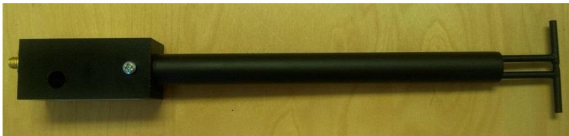
Figure 1 – MVG COMOSAR Validation Dipole
