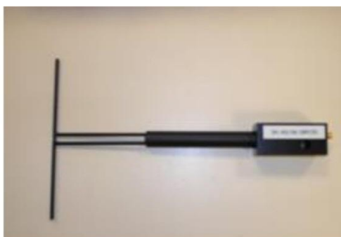
Figure 1 – Satimo COMOSAR Validation Dipole
