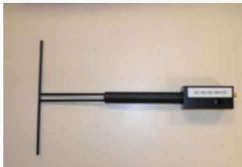
Figure 1 – Satimo COMOSAR Validation Dipole
