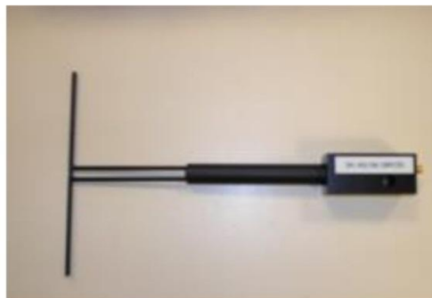
Figure 1 – Satimo COMOSAR Validation Dipole
