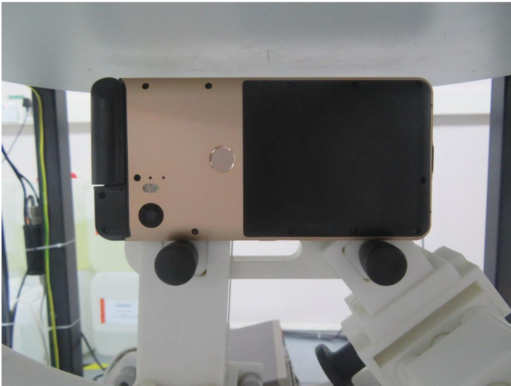
10mm body-worn Left Side Setup Photo (hotspot)
