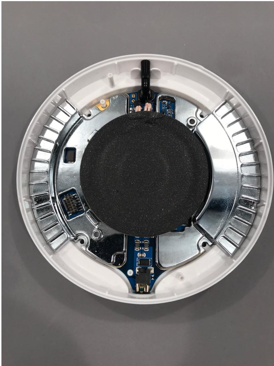
Coil foam removed to expose the antenna
