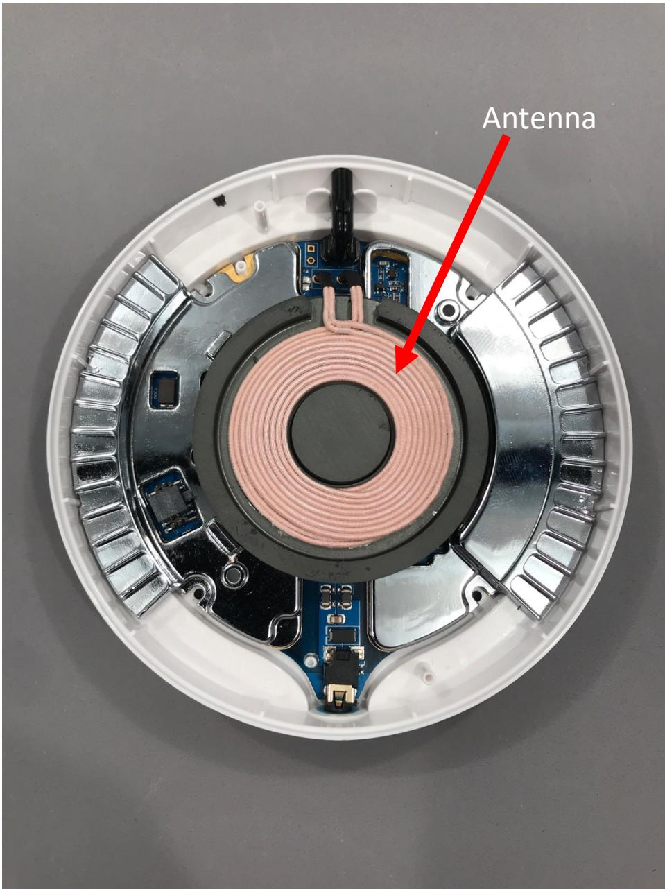
PCBA with attached coil
