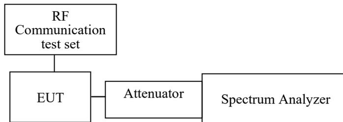
Note: The path loss from EUT to Spectrum Analyzer has included in the result.
