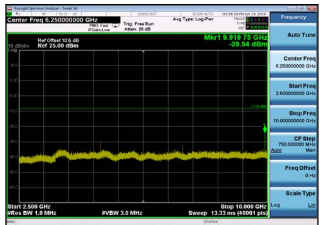
Conducted Emission: 8DPSK,2480,3DH5 ,2500MHz~10000MHz
