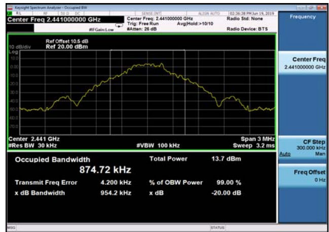
20dB Bandwidth: DQPSK,2402MHz,2DH5
