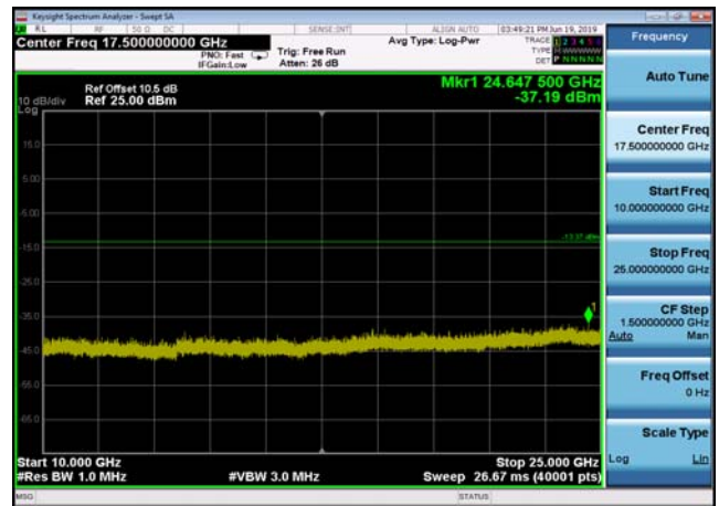
Conducted Emission: DQPSK,2480,2DH5 ,30MHz~2310MHz
