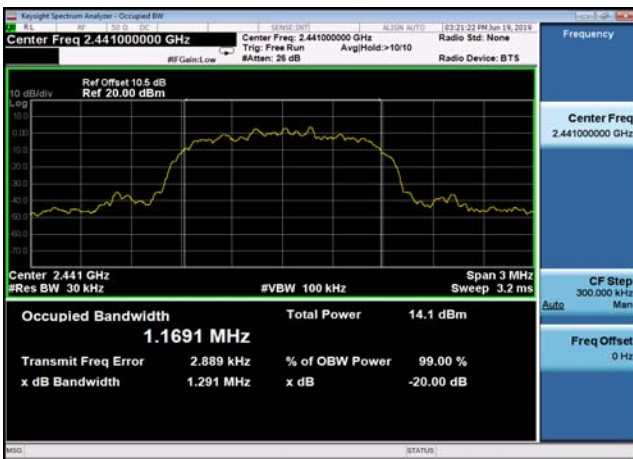
20dB Bandwidth: DQPSK,2441MHz,2DH5
