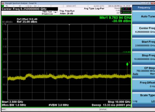
Conducted Emission: 8DPSK,2441,3DH5 ,Band Edge HoppingOFF
