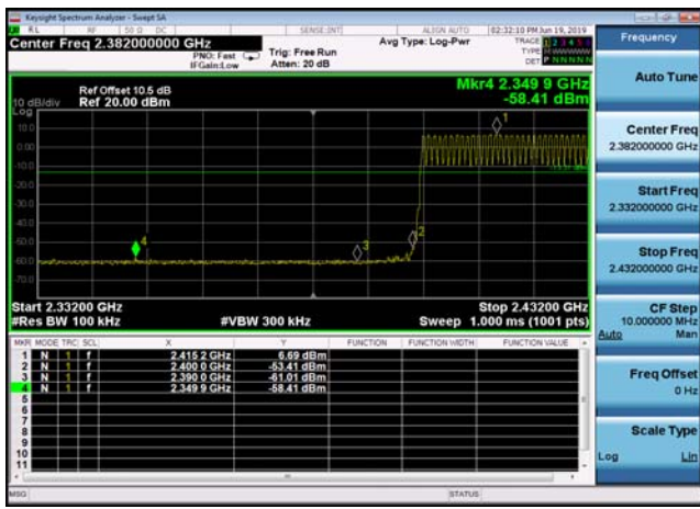
Conducted Emission: DQPSK,2402,2DH5 ,Band Edge
