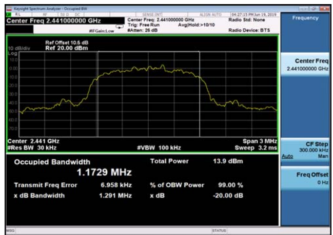
20dB Bandwidth: 8DPSK,2441MHz,3DH5
