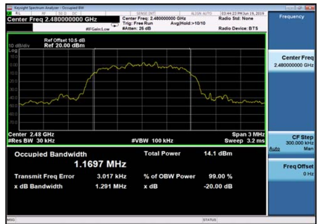
20dB Bandwidth: DQPSK,2480MHz,2DH5
