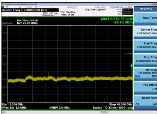
Conducted Emission: DQPSK,2480,2DH5 ,Band Edge HoppingOFF
