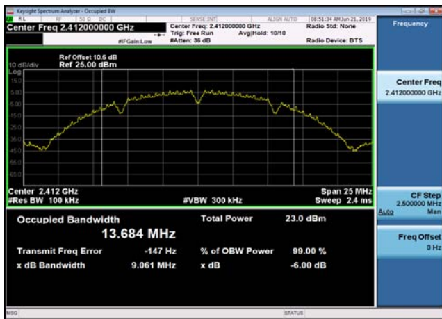
6dB Bandwidth-802.11b,2437MHz,Ant0
