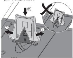
> Slide the phosphor storage plate out of its barrier envelope downwards into the device until the phosphor storage plate is automatically drawn in.
