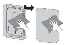
> Allow the barrier envelope and phosphor storage plate to dry completely.
