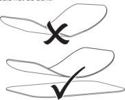
> Do not scratch the phosphor storage plates. Do not subject the phosphor storage plates to pressure from hard or pointed objects.
