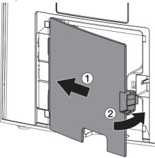
When operating the device, the cover on the rear must be mounted.
