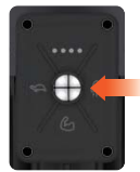
Please long press the power button of the main body to complete power on/off.
