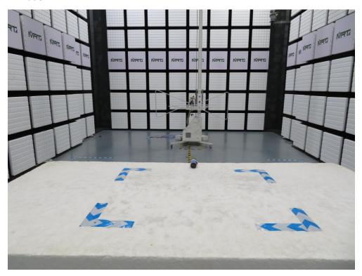
Description: Radiated Spurious Emission Test Setup for Above 1GHz Mode 1
