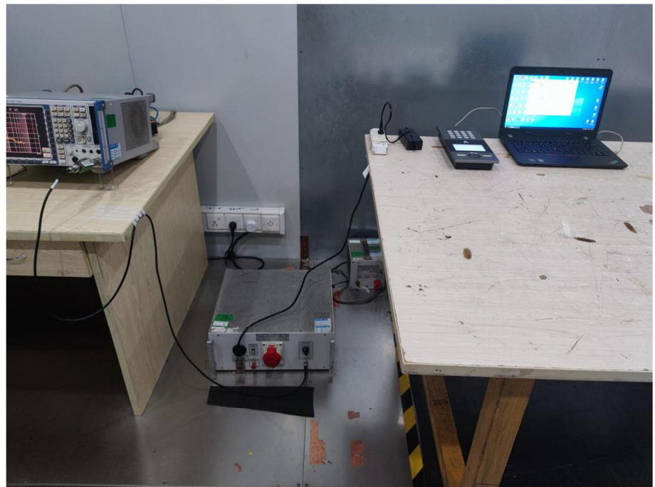
Conducted Emission Test Setup
