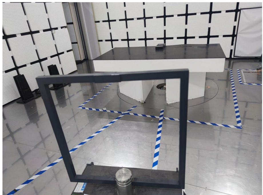
Radiation Emission Test Setup (Below 30MHz)
