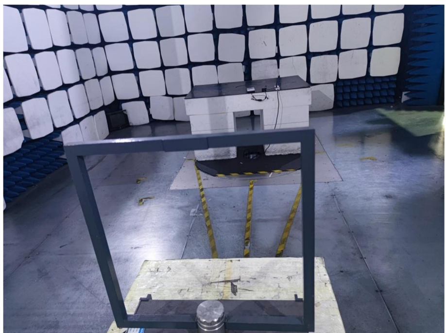
Radiation Emission Test Setup (Below 30MHz)
