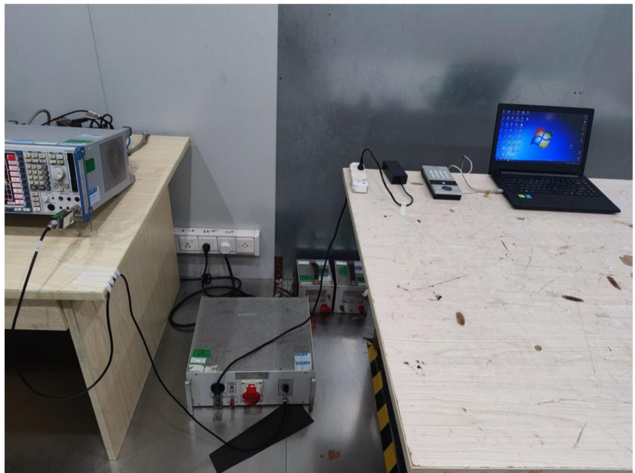
Conducted Emission Test Setup
