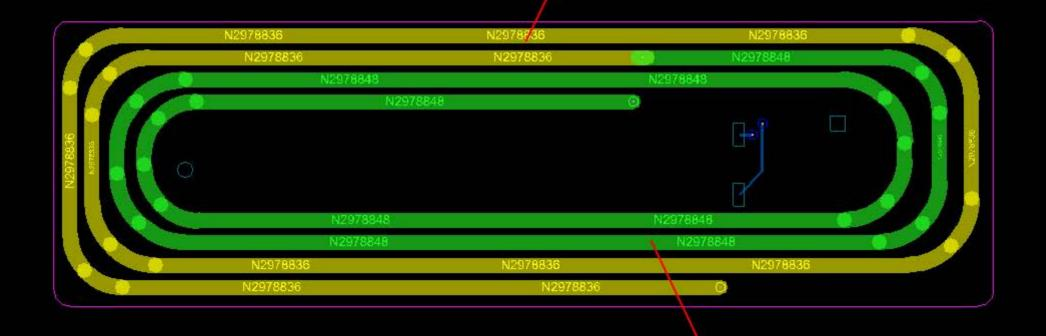
Green line length is 233.76mm, width is 1.0mm, the thickness is 10Z.
