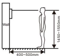
The camera should be 1450~1550mm above the ground.
