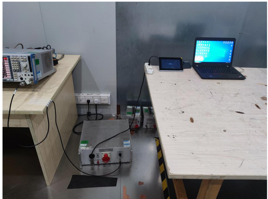
Conducted Emission Test Setup
