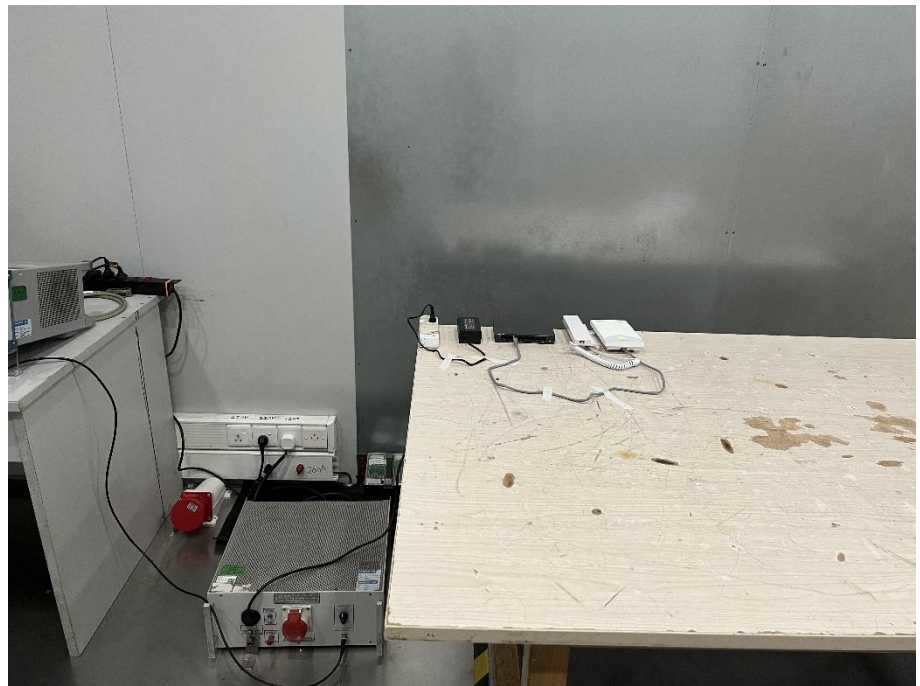
Conducted Emission Test Setup
