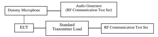
Setup Block Diagram for Audio Frequency filter:
