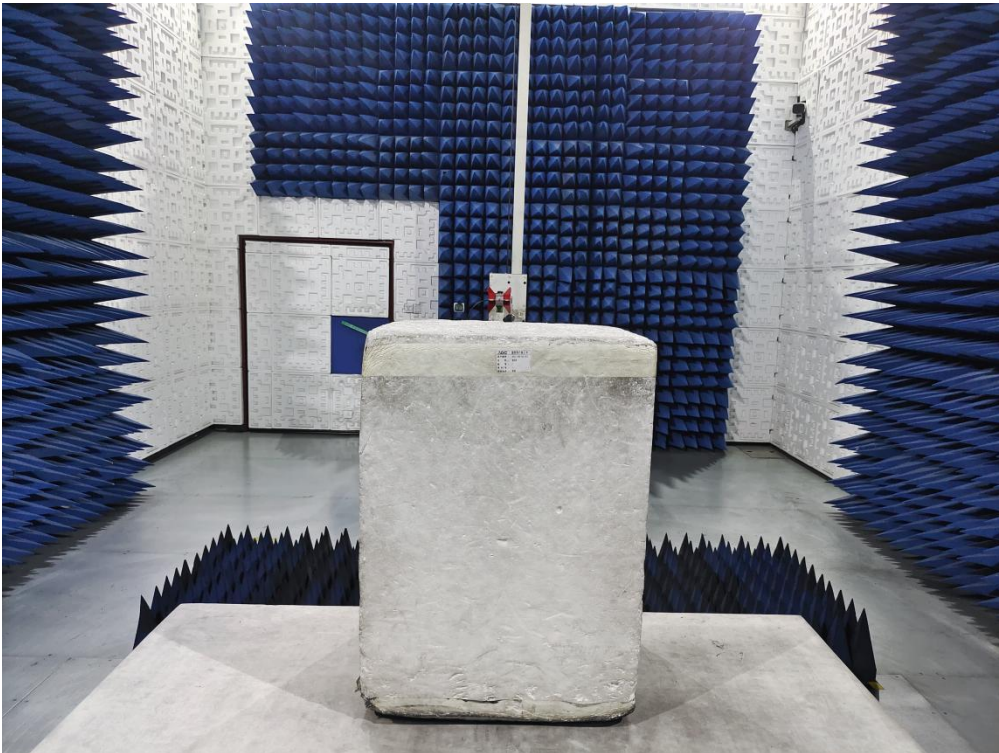
RADIATED EMISSION TEST SETUP ABOVE 1GHz
