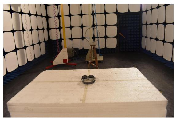
3. Radiated emission (9KHz-30MHz)
