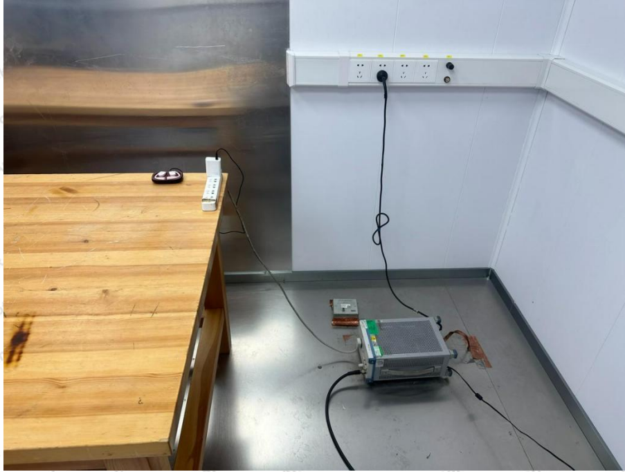
Conducted Emission at AC power line
