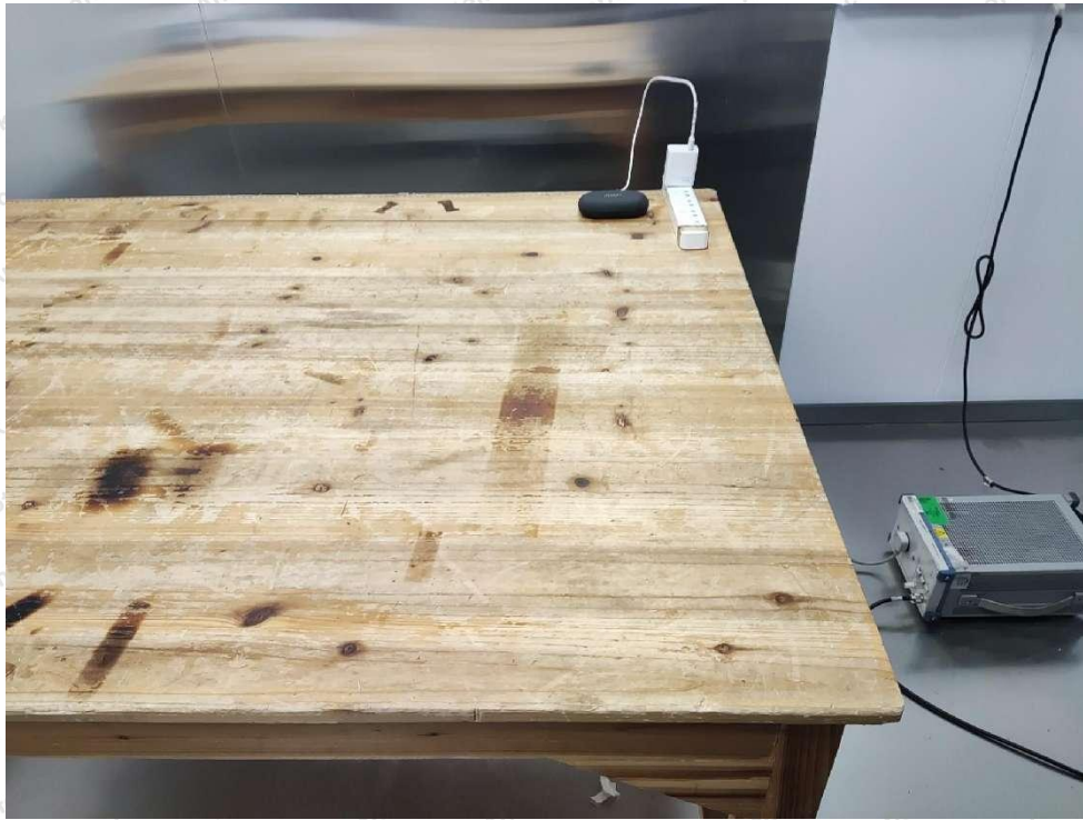
Photo of Conducted Emission Measurement
