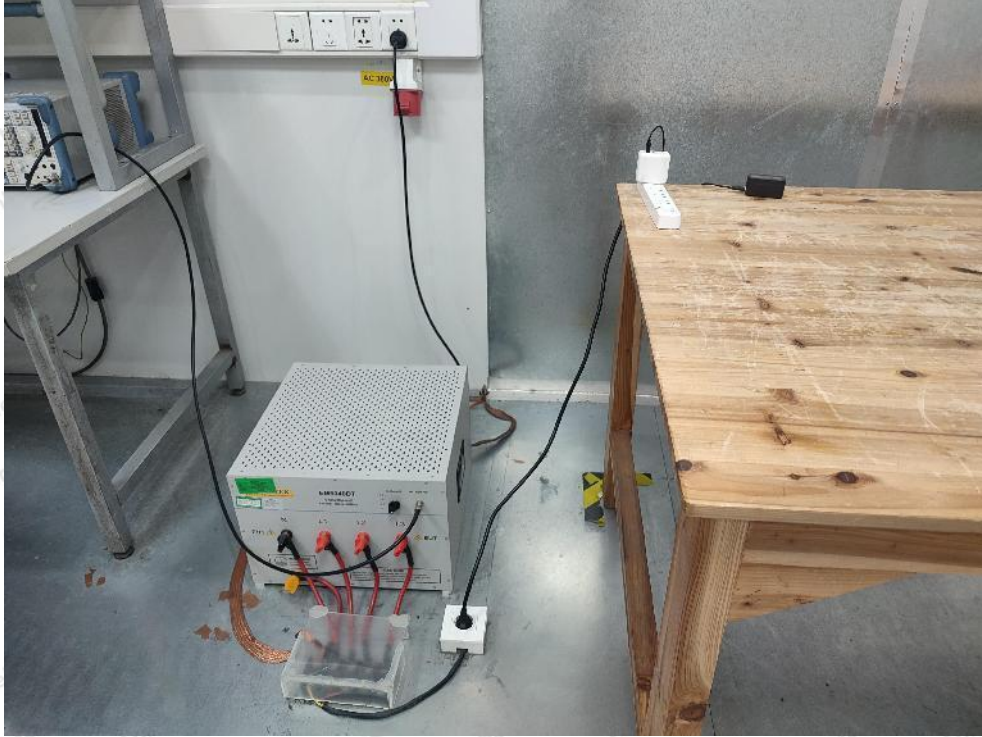
Photo of Conducted Emission Measurement
