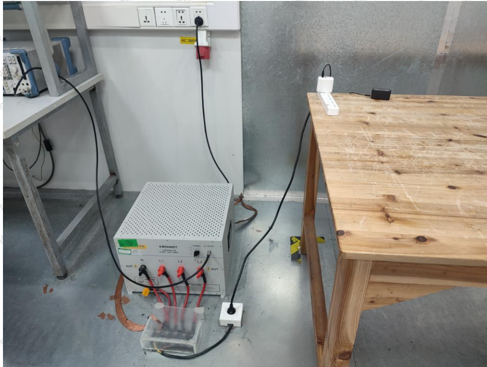
Photo of Conducted Emission Measurement
