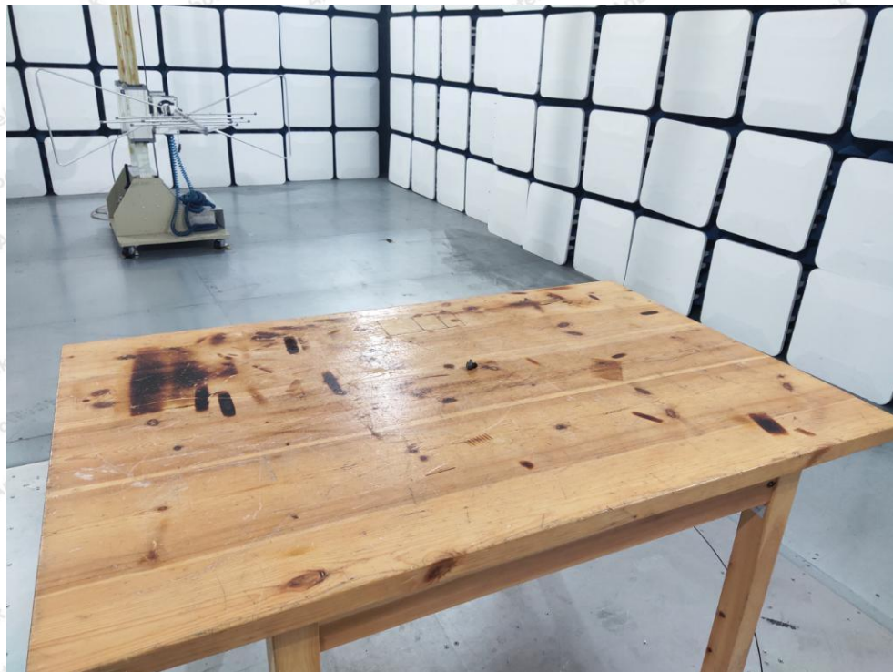
Photo of Radiation Emission Test
