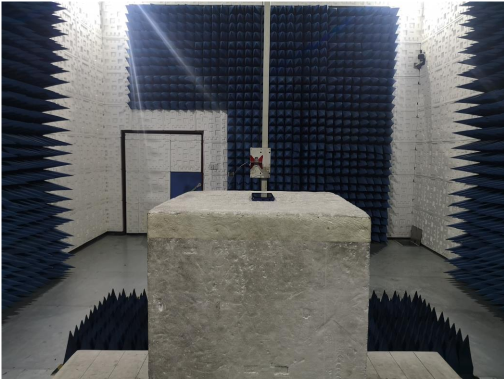
RADIATED EMISSION TEST SETUP ABOVE 1GHZ
