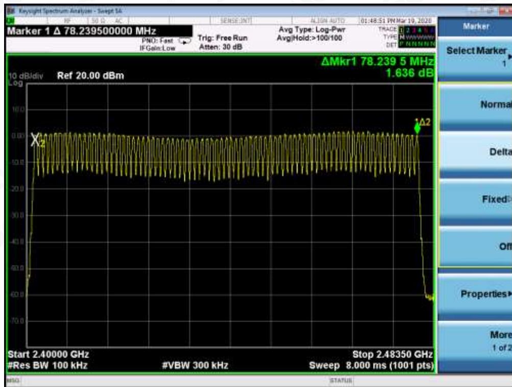
TEST PLOT FOR NO. OF TOTAL CHANNELS
