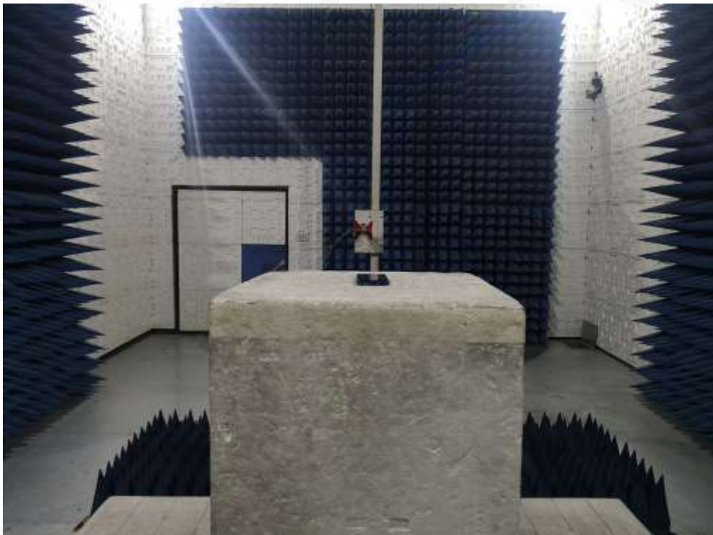
RADIATED EMISSION TEST SETUP ABOVE 1GHZ
