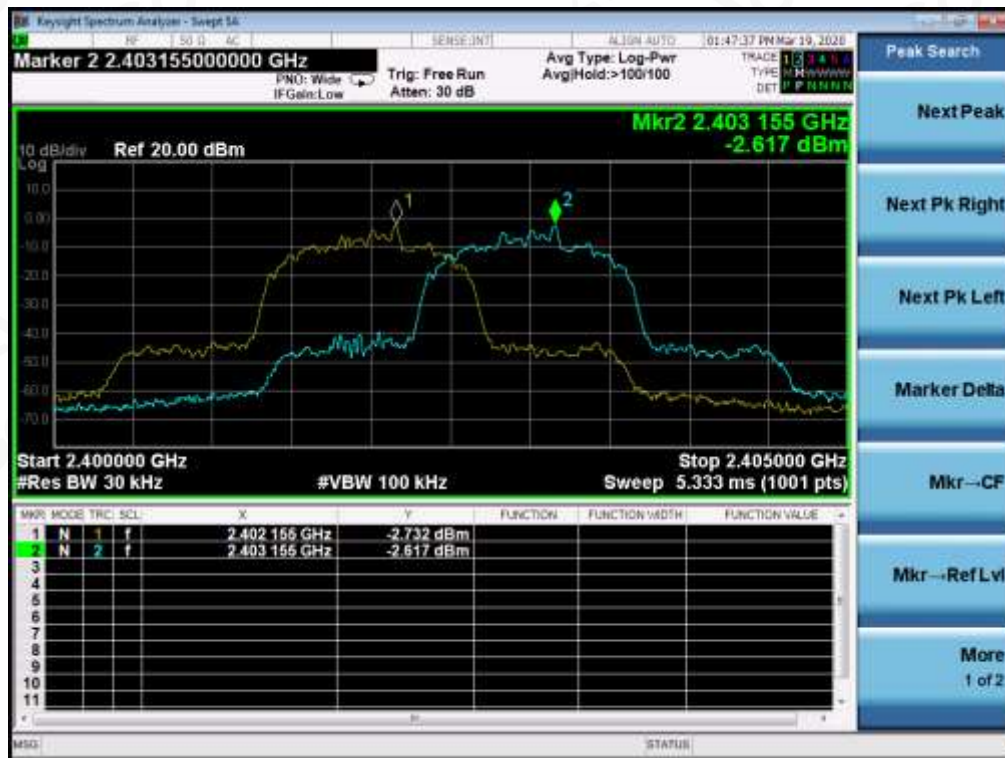
TEST PLOT FOR FREQUENCY SEPARATION
