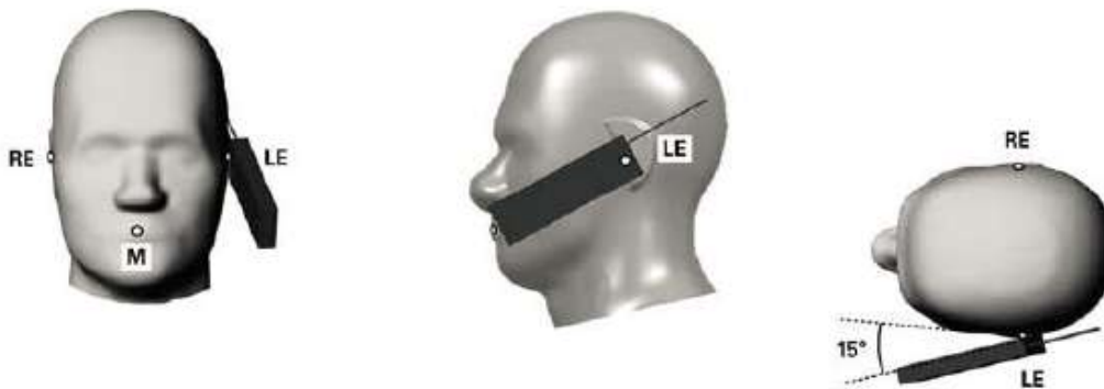
Fig.11.4 Illustration for Tilted Position
