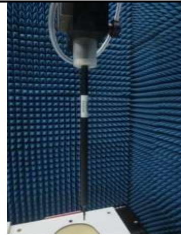
Fig.8.2 Photo of E-Field Probe
