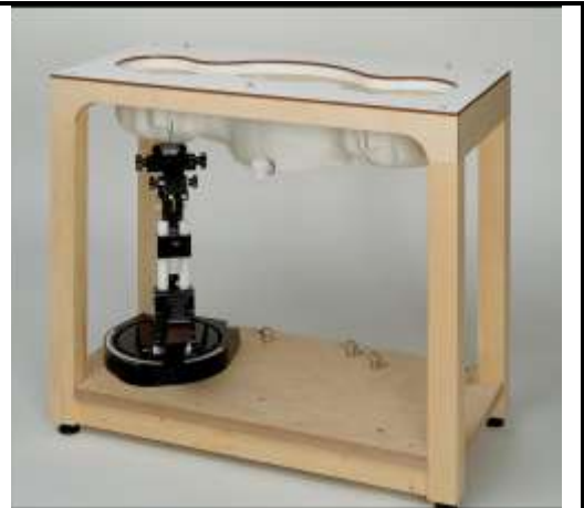
Fig. 8.7 Photo of SAM Twin Phantom
