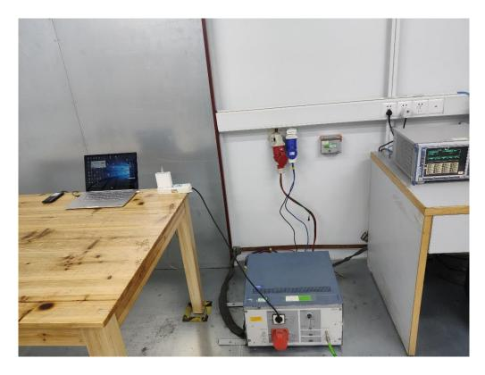
FCC RADIATED EMISSION TEST SETUP
