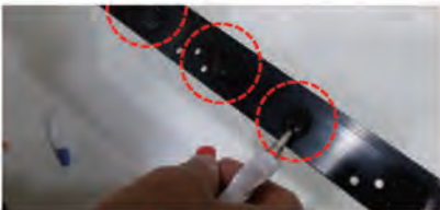
fig.4 Squeeze enclosed adhesive A and B as show in figure at same amount.
