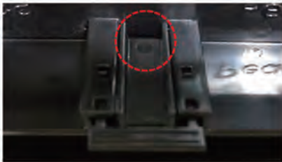
Fig.2 There is accessory for removal and mount at handle side.
