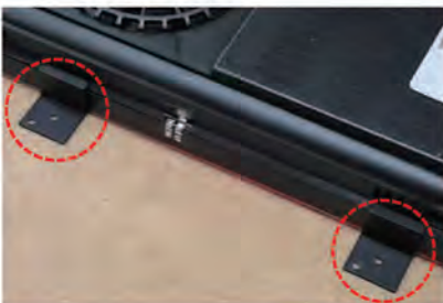
Fig.3 Stick bracket to side of Under Range, and then fix screws on 4 points with screw driver.
