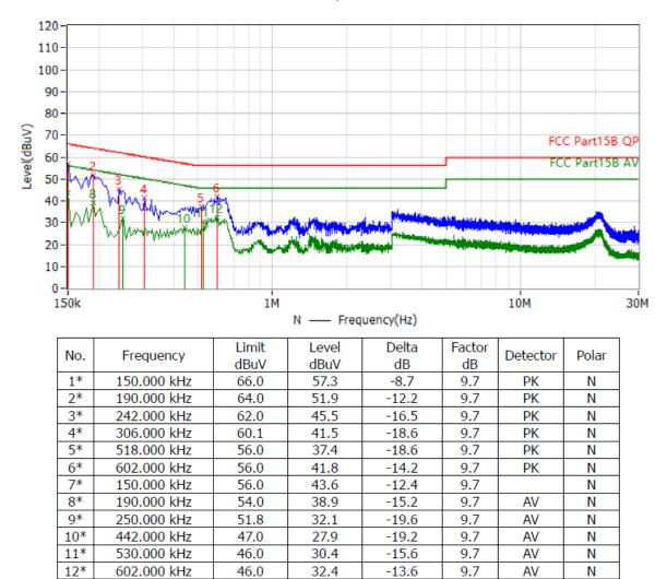
Note: All modes and channels have been tested and only the GFSK 2441MHz mode with the worst data is listed.
