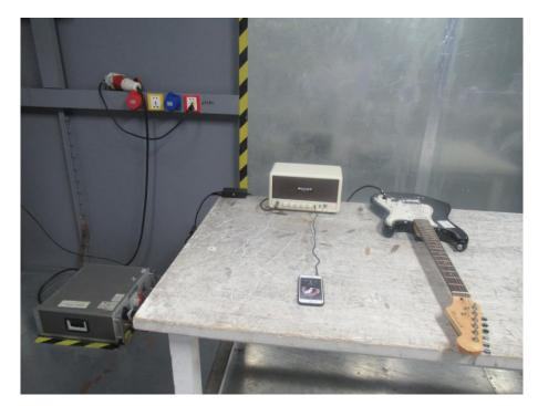
Photos of Conducted Emission test
