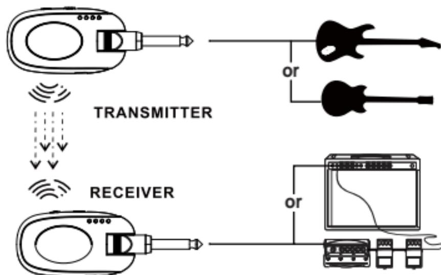
1. Transmitter plugs into the Guitar (you instruments), the receiver plugs into the effects pedal, AMP, Audio, etc.
