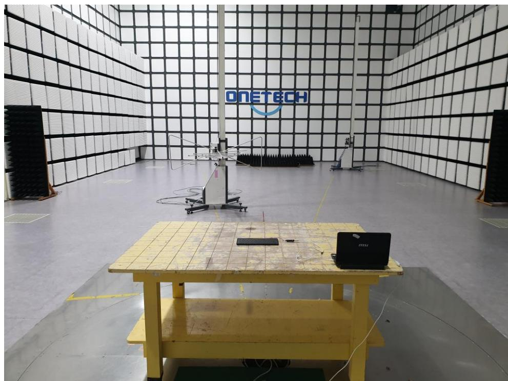
**- Radiated Emission Test (Above 1 GHz)**
