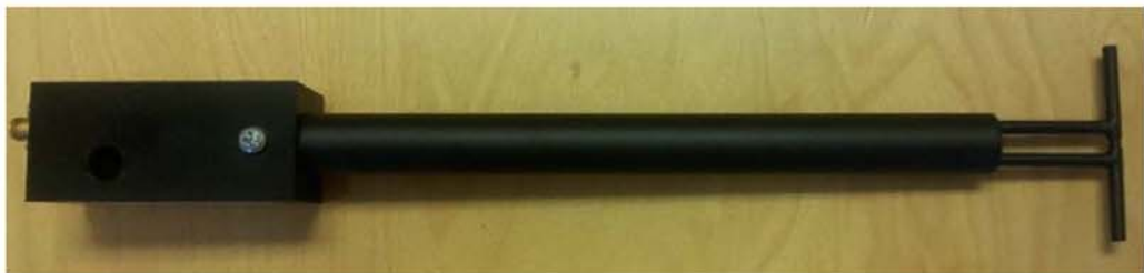
Figure 1 – MVG COMOSAR Validation Dipole
