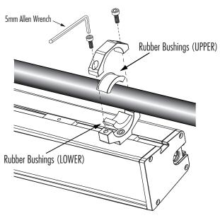
Two rubber bushing sizes are provided. The thinner bushings are for RZR vehicles with 1.75 inch ROPS tubing. The thicker bushings are for ACE and ATV vehicles with 1.5 inch tubing.
