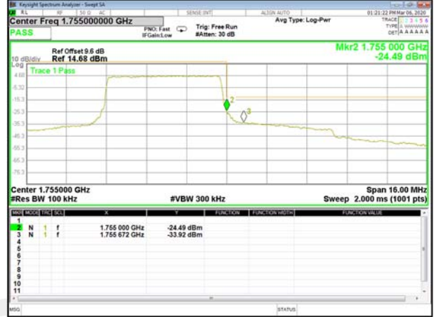
16QAM_5M_Lower_Band edge_Full-RB
