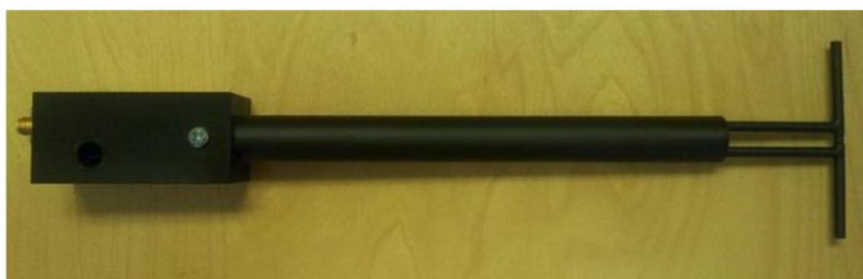
Figure 1 – MVG COMOSAR Validation Dipole
