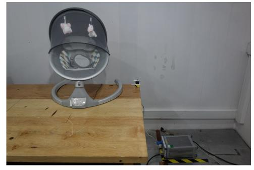
**1.2 Radiated Spurious Emissions Test Setup** Below 1GHz
