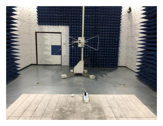
RADIATED EMISSION TEST SETUP ABOVE 1GHZ
