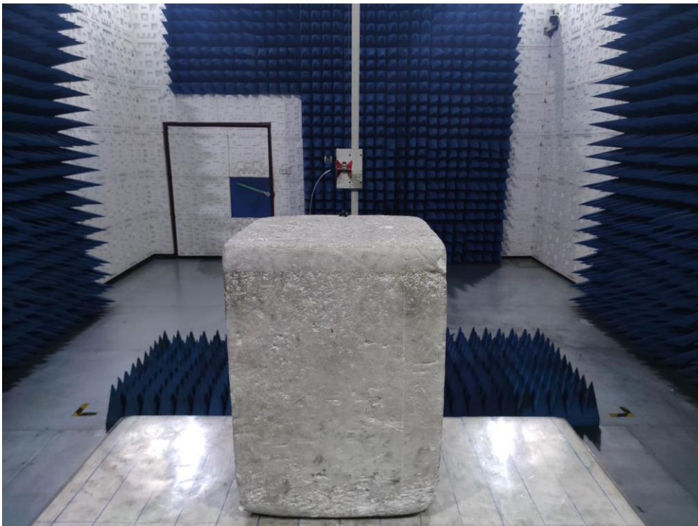
RADIATED EMISSION TEST SETUP ABOVE 1GHz
