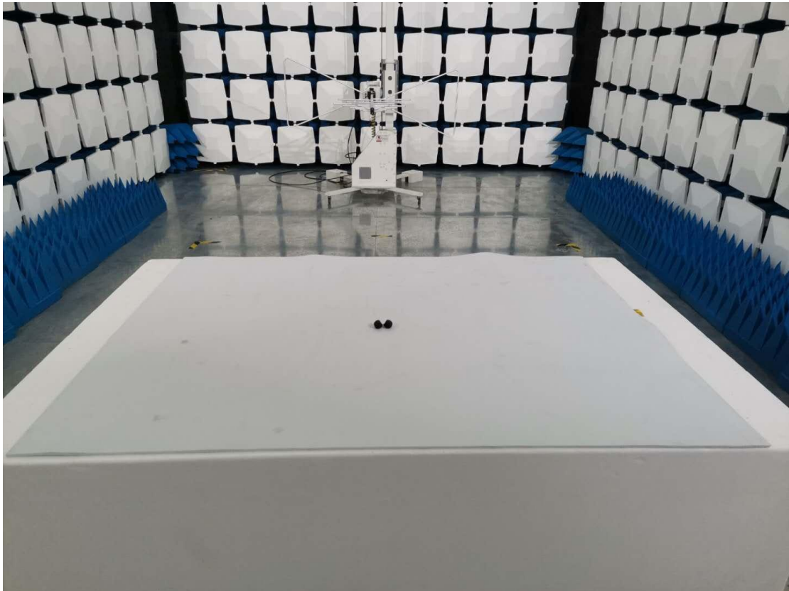
Blow 1GHz for radiated emission test setup
