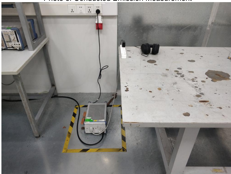
FCC ID: 2ATQ9-M98 Photo of Conducted Emission Measurement
