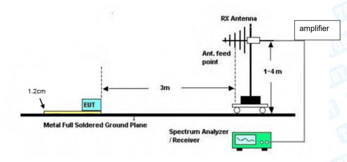
Below 1000MHz Test Setup
