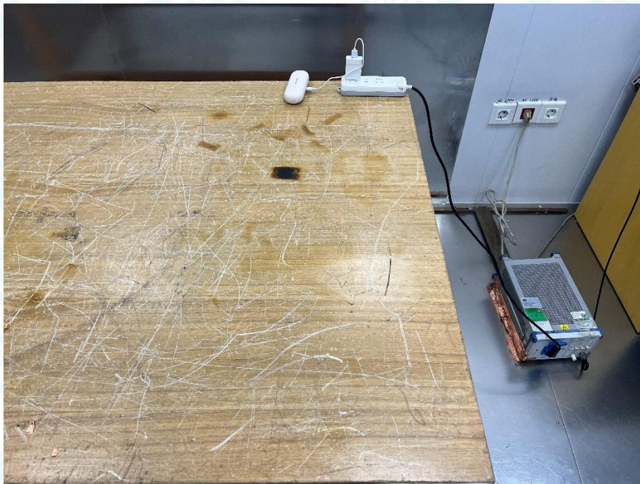
Photo of Setup for Conducted Emission
