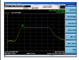
Power spectral density plot on channel 13
