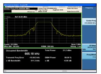
6dB Bandwidth plot on channel 24
