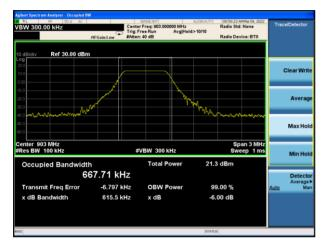
6dB Bandwidth plot on channel 13
