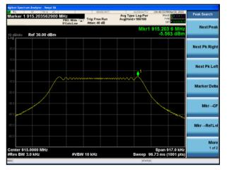
Power spectral density plot on channel 24
