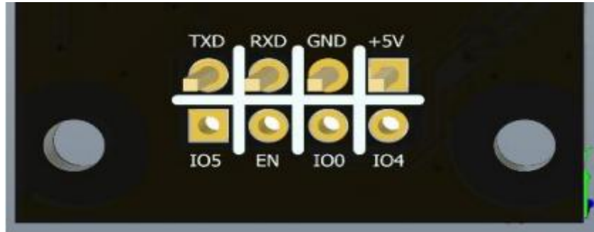
ESP-15F Pin diagram
